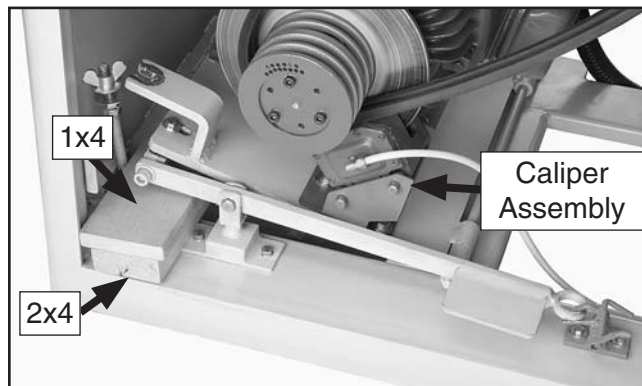
Figure 70. 2x4 positioned between frame and motor.
